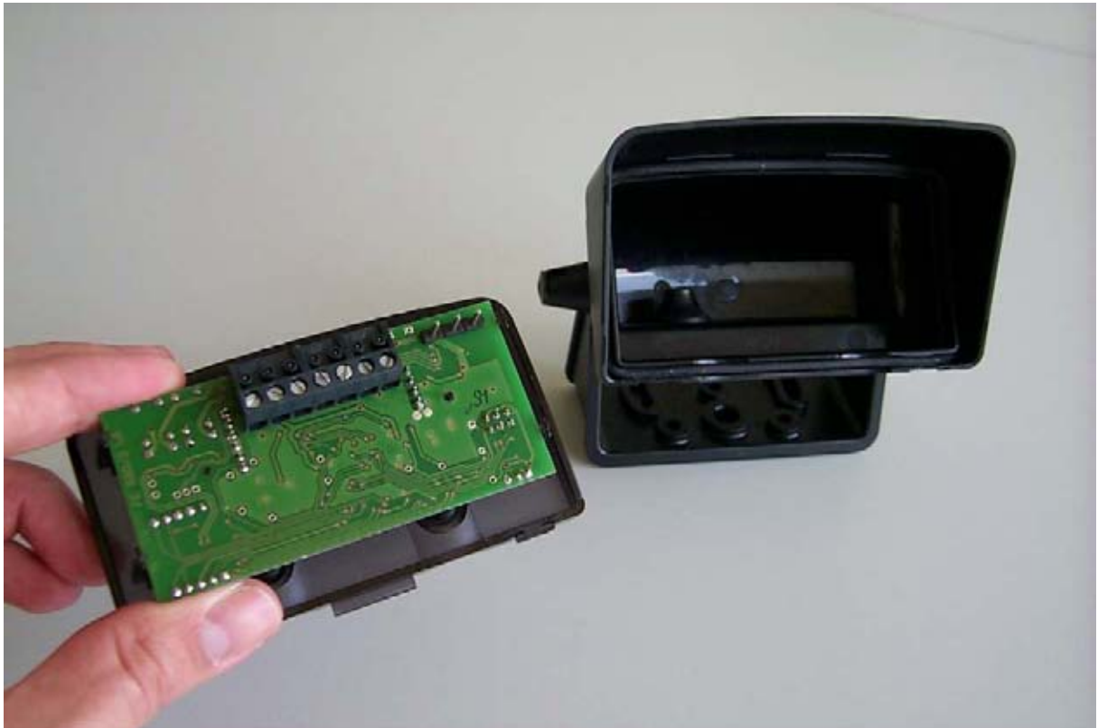
The electronic component is equipped with a clamp block for easy installation.
